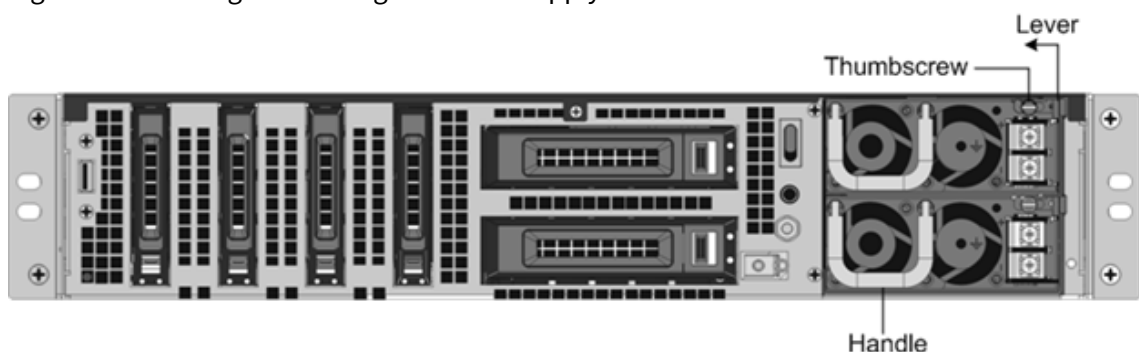
Figure 3. Removing the Existing DC Power Supply
