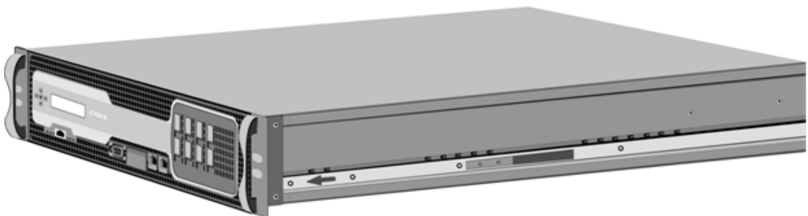
Figure 1. Attaching inner rails
